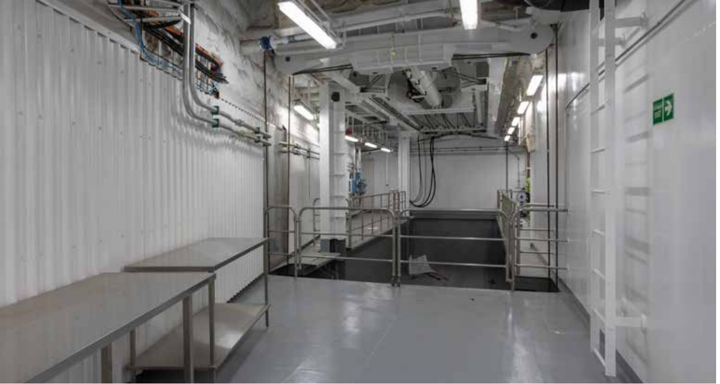
The void for the hydraulic hoistable catering-ramp on deck 2.
