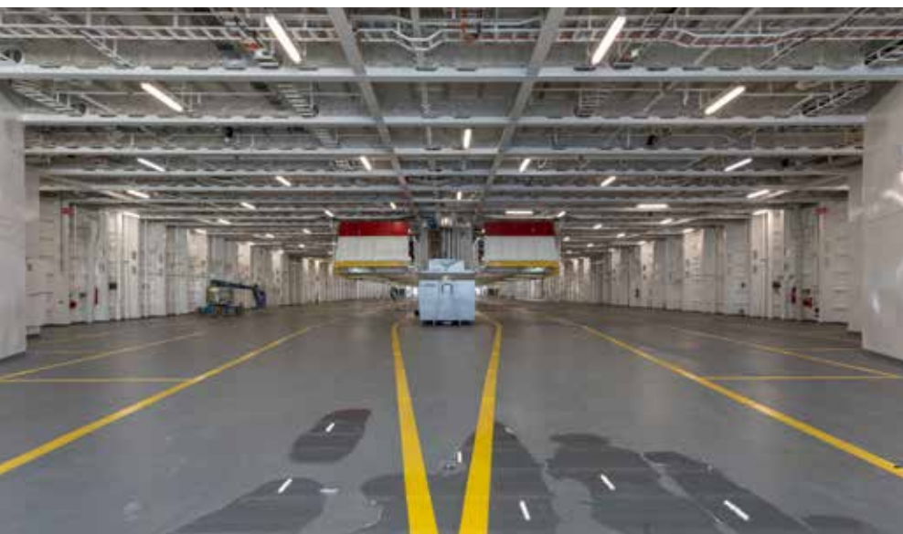
Another view of deck 5 with the hydraulic hoistable decks on both sides of the casing.
