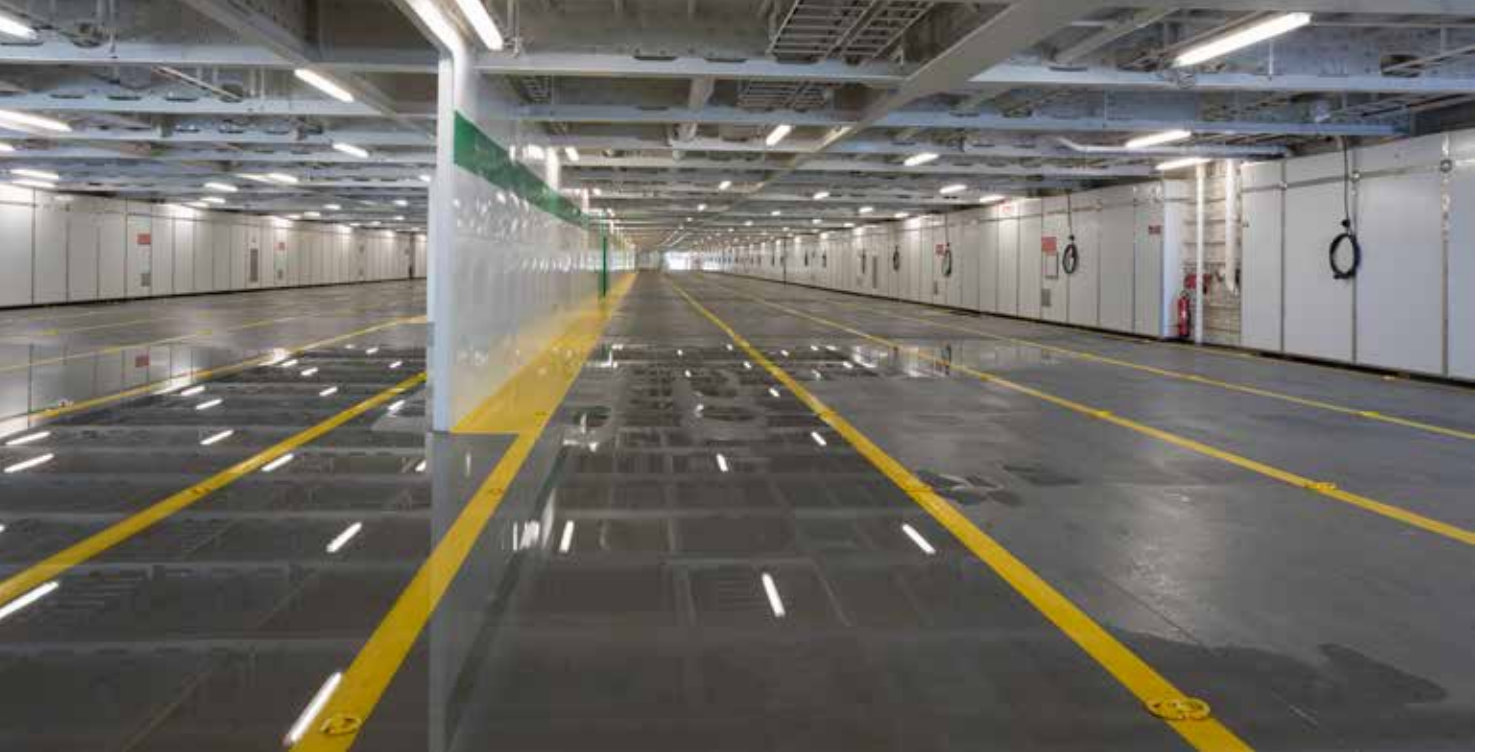
CBG Systems has delivered lightweight panelised A60 structural fire protection to the bulkheads between the car deck 7 and the outside MES-areas in both sides. There are 20 charging points for EVs on Deck 7.
